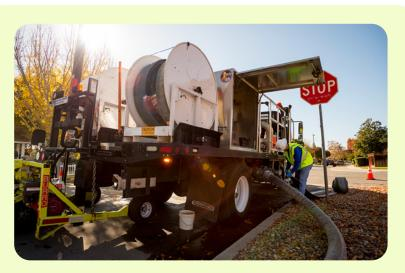
Flushing Truck – SJW's flushing truck saves about 30,000 gallons of water per flush compared to traditional flushing methods. That is a savings of approximately 6 million gallons per year. Using Neutral Output Discharge Elimination System (NO-DES) technology, effective flushing and sediment removal is obtained with minimal water waste. SJW is improving water quality while saving water.
